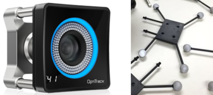
Figure 4.2: Optitrack IR camera and IR markers.
