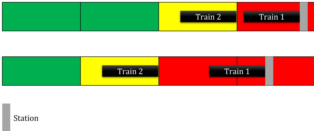
Figure 5.17: Influence on coloured signalling of the station positioning inside the block
