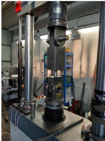
Figure 2-37: Prototype installed on the testing machine
