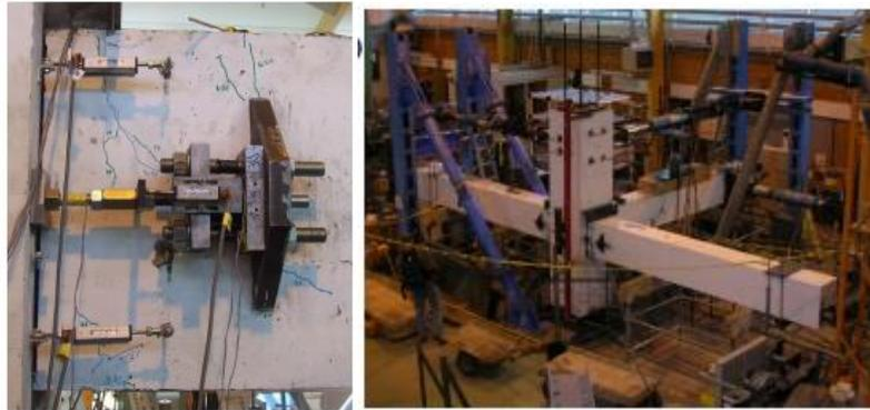
Figure 2-24: Left: lead extrusion damper externally mounted to the seismic beam; right: photograph of test specimen [73]
