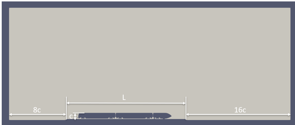
Figure 3.4. Minimum distances for the models according to [12]
