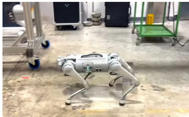
Figure 2.4: Quadruped robot used for visual inspection and interventions in remote and inaccessible areas. (Retrieved from [8]).
