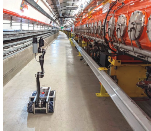
Figure 2.3: MIRA robot: a compact autonomous mobile robot used for radiation surveying, inspection, and remote operations in the SPS (Super Proton synchrotron) tunnel. (Retrieved from [8]).
