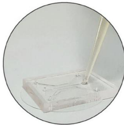
Figure 3.2: Representative picture of the fabricated PDMS microfluidic device bonded to a glass coverslip, shown during loading via pipette [100].
