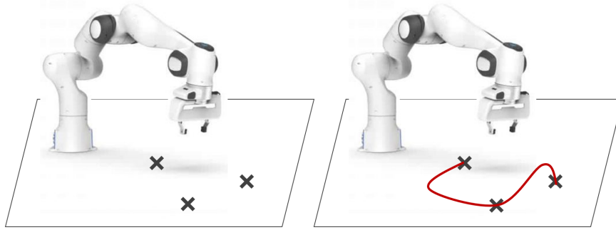
Figure 2.8: Position Control on the left, where only three intermediate points are given VS Path Control on right, where all the path is provided (red)
