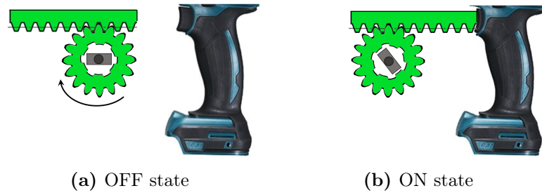
Figure 4.13: Trigger activation, rack-pinion mechanism
