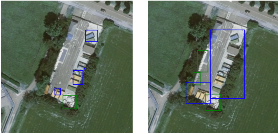
Figure 7.15: CAMs qualitative analysis for Weakly Supervised Object Detection - Second example (On the left the derived prediction and on the right the ground truth)
