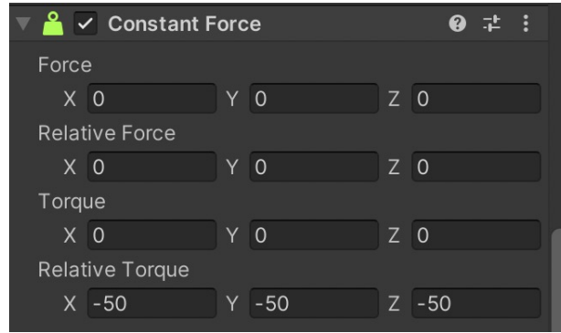
Figure 13: one sample of the force component used with the relative torque parameter
