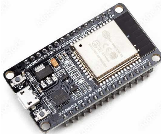
Figure 3.3: ESP32-WROOM-32 Pin Layout (Top View) [15]
