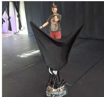
Figure 3.1: The robot Blackwing at work for the project My Robot Body in 2024. Controlled by a participant with sound and motion of the head and wrist [14].
