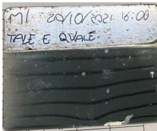
Figure 93 - Metal sheet of the Hull cell test of 20/10/2021
