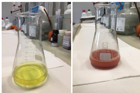
Figure 27 - From left to right: diluted zinc bath + potassium chromate, previous solution titrated with \text{AgNO}_3
