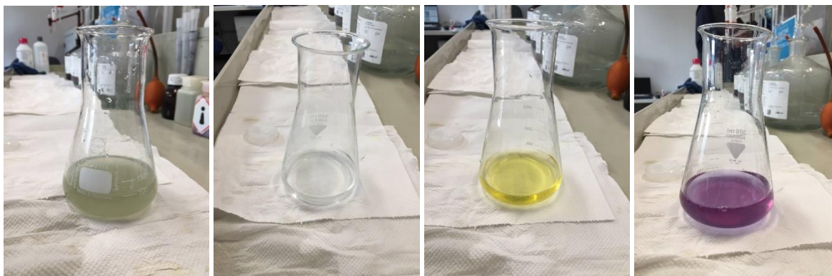
Figure 29 - From left to right: pickling bath, diluted pickling bath, diluted pickling bath + blü di bromofenolo, previous solution titrated with NaOH
