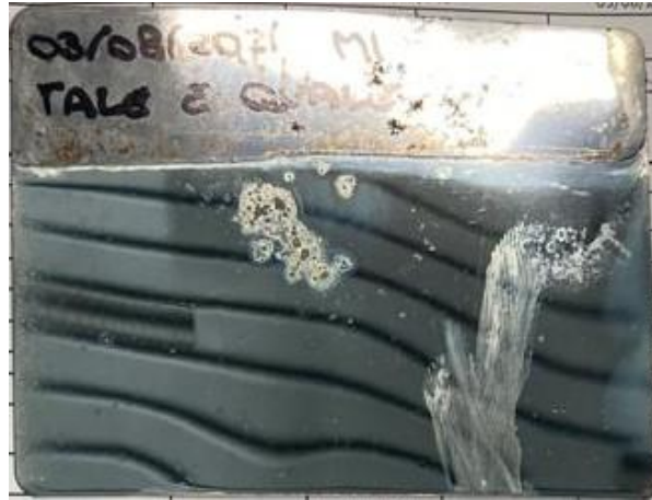
Figure 90 - Metal sheet of the Hull cell test of 03/08/2021
