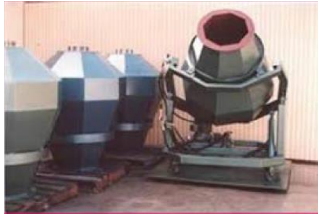
Figure 6 - Rotating reactor for mechanical zinc deposition [4]
