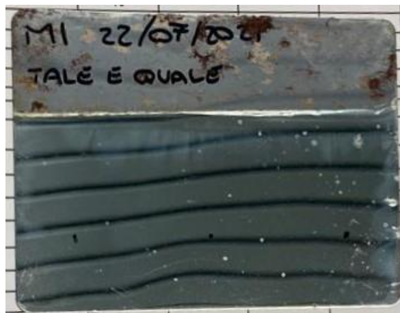
Figure 87 - Metal sheet of the Hull cell test of 22/07/2021
