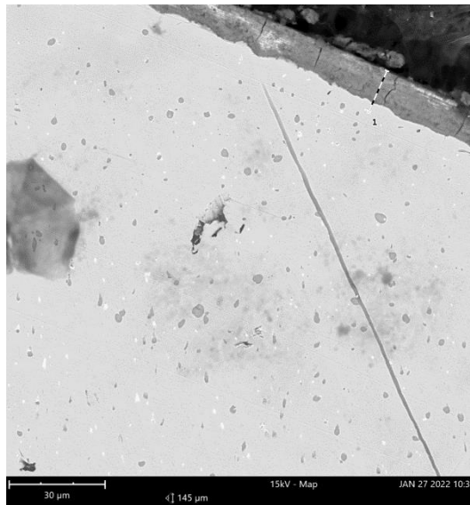
Figure 101 - Section of C8 sample with indicated the direction (black and white line) of the analysis of the zinc layer
