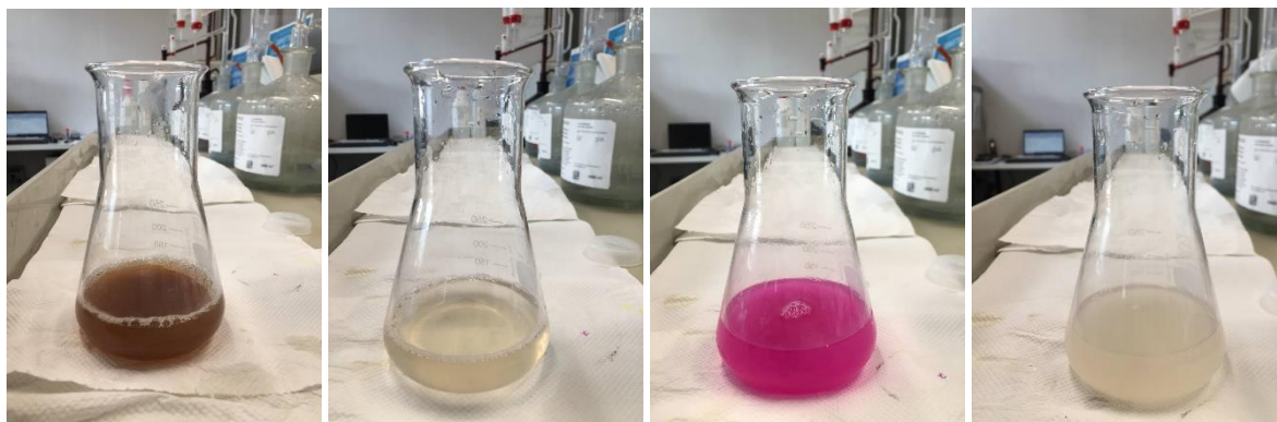
Figure 30 - From left to right: chemical degreasing bath, diluted chemical degreasing bath, diluted chemical degreasing bath + phenolphthalein, previous solution titrated with HCl
