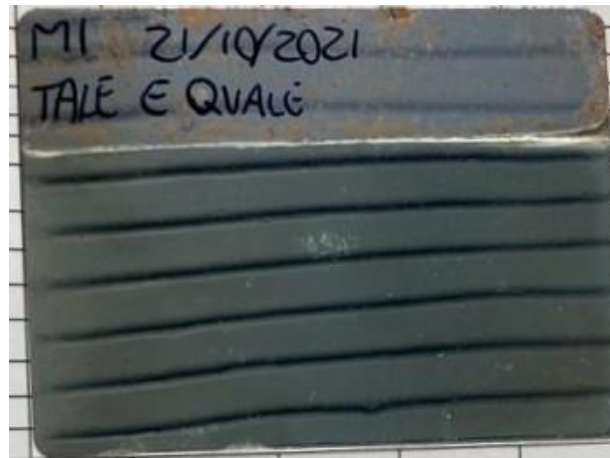
Figure 94 - Metal sheet of the Hull cell test of 21/10/2021
