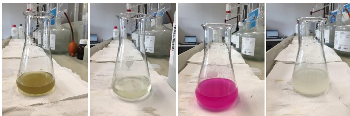
Figure 31 - From left to right: electrolytic degreasing bath, diluted electrolytic degreasing bath, diluted electrolytic degreasing bath + phenolphthalein, previous solution titrated with HCl
