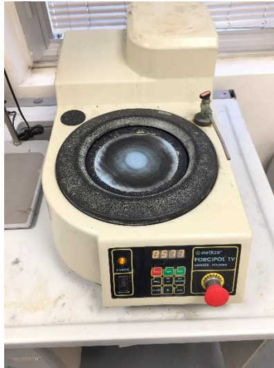
Figure 40 - Lapping instrument Mekton Forcipol 1V
