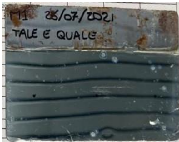
Figure 88 - Metal sheet of the Hull cell test of 26/07/2021
