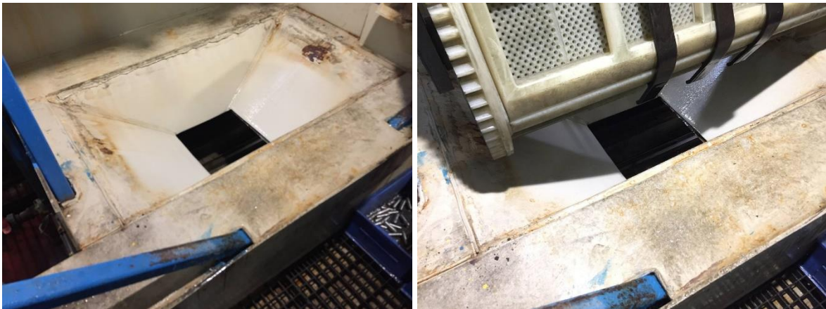
Figure 21 - Funnel used to transfer the parts from one type of barrel to the other
