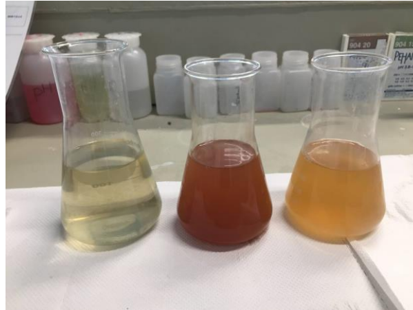
Figure 19 - From left to right: zinc bath, zinc bath + \text{H}_2\text{O}_2 , filtered zinc bath + \text{H}_2\text{O}_2
