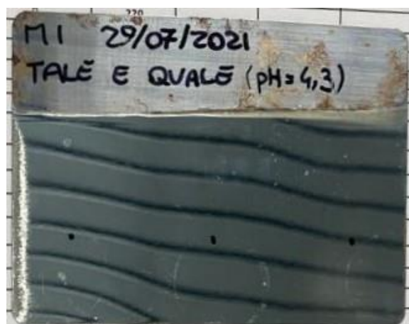
Figure 89 - Metal sheet of the Hull cell test of 29/07/2021
