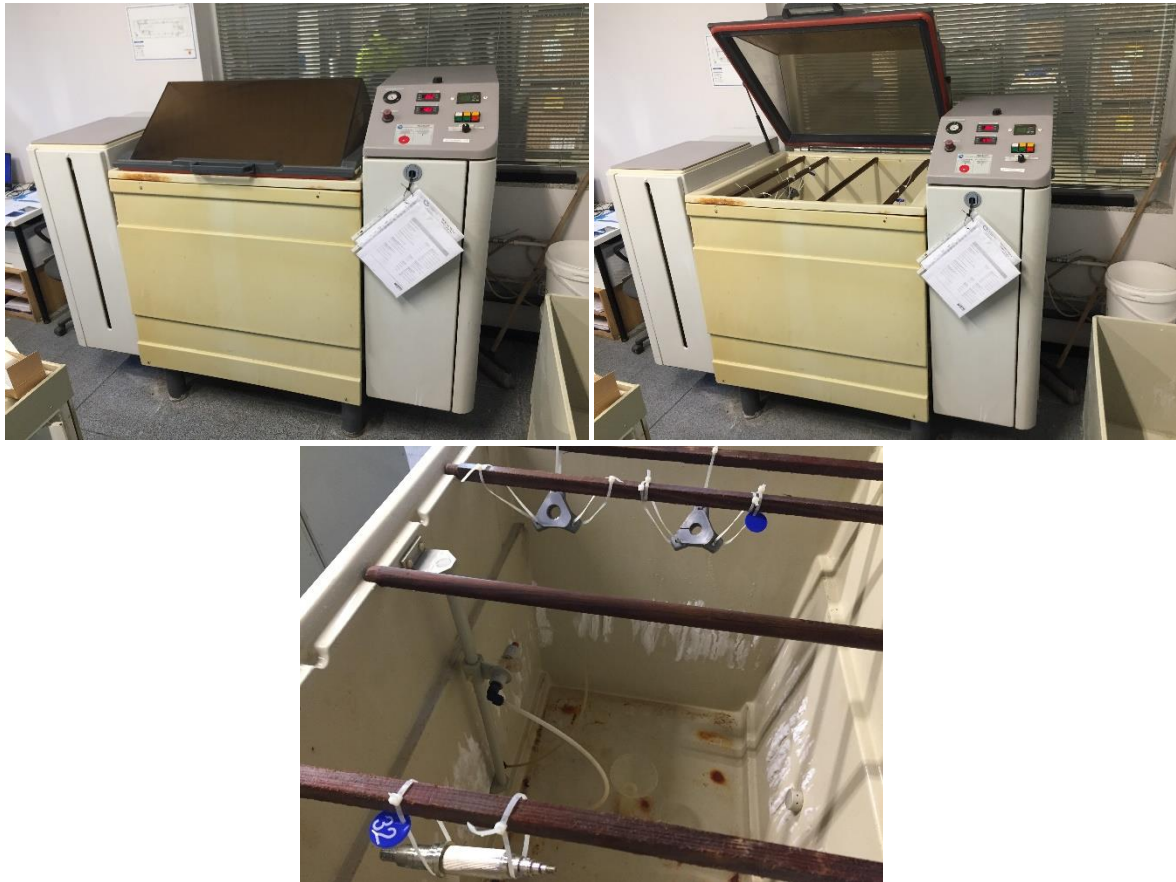
Figure 38 - Salt spray machine Angelantoni DCTC600
