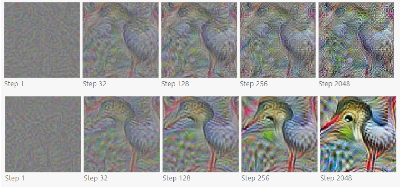
Figure 5.2: Images generated without imposing transformation robustness (top) compared with same images generated imposing transformation robustness. Note how high frequency noise disappear when transformations are introduced.
