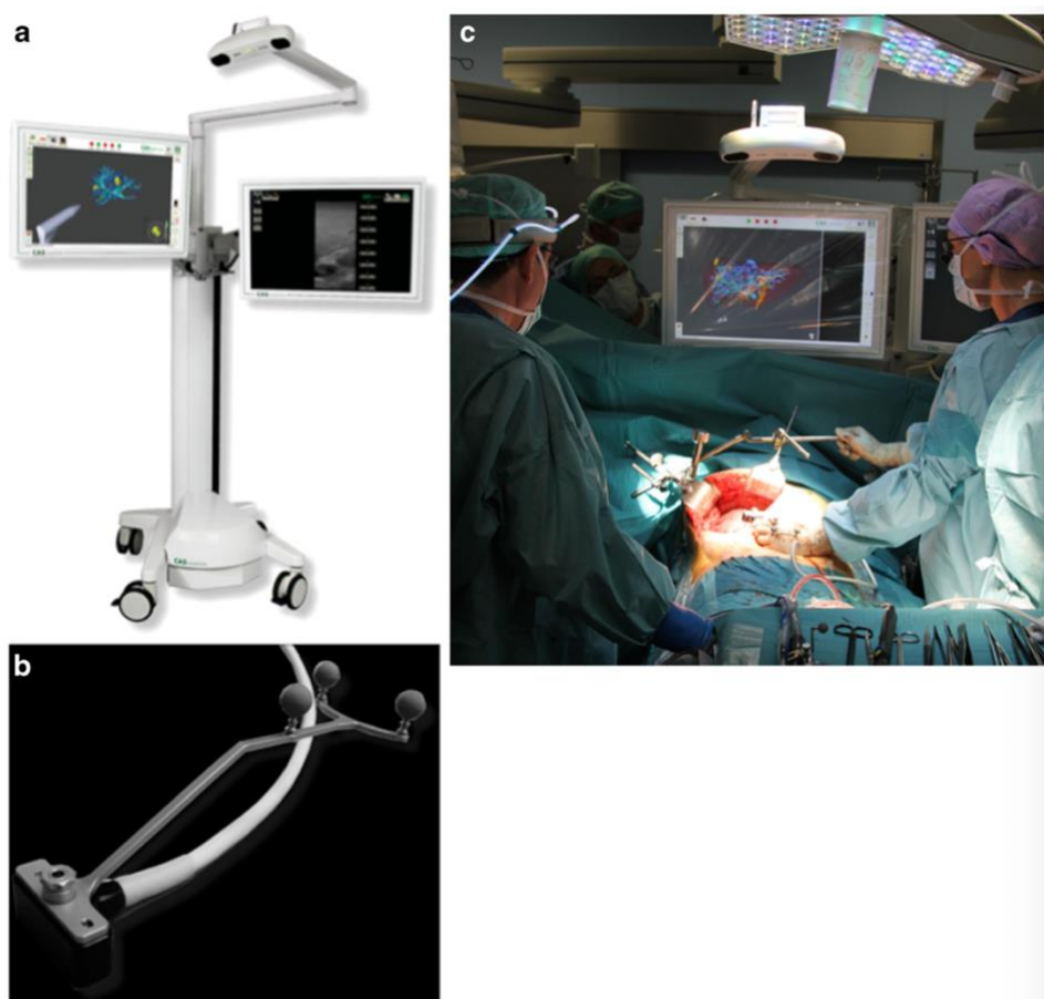
Figure 40 (a) 3D reconstruction of the CT-scan is shown on the left monitor and the integrated US for patient-to- image registration is displayed on the right monitor. (b) integrated and navigated sonography probe. (c) set up of surgical navigation system [98].
