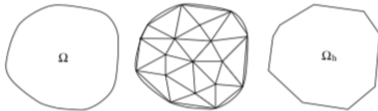
Figure 1.7: Example of meshing a non polygonal domain [Quarteroni, 2013].
