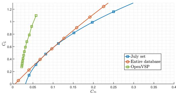
Figure 6: Drag polar comparison: fitting of the datasets vs. OpenVSP prediction.
