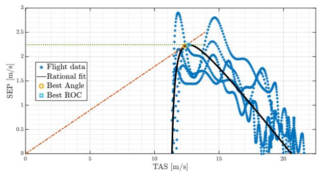
Figure 7: *SEP* fitting curve and associated performance.
