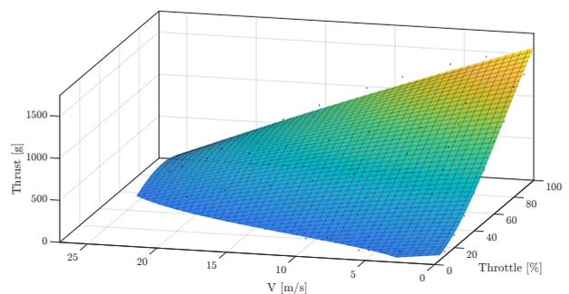
Figure 3: APC 10x55MR wind tunnel data fit carpet plot.
