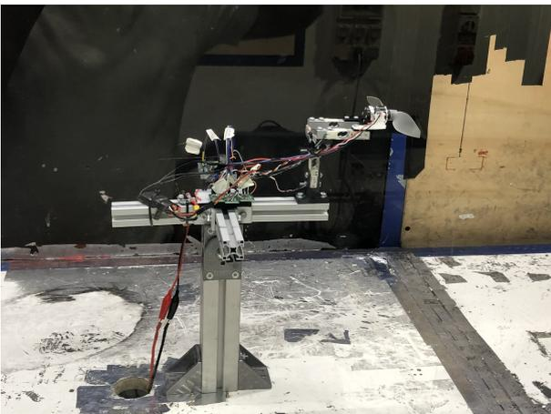
Figure 2: Test bench configuration with the APC 10x55MR mounted for wind tunnel testing.
