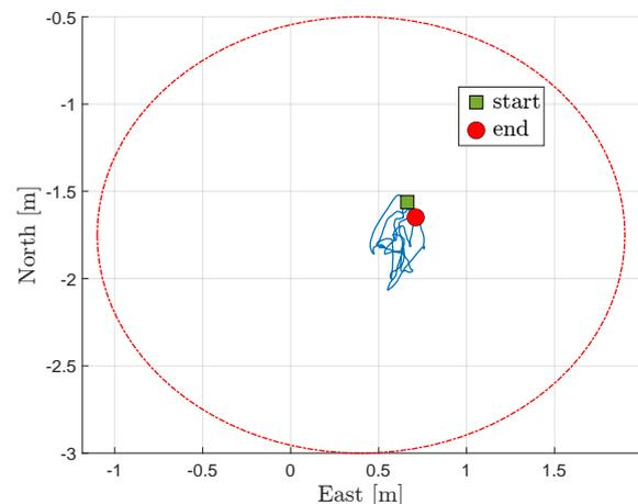
Figure 4: Trajectory during hover with GPS module on the right wing, red dash-dot curve represents position drift before the modification.
