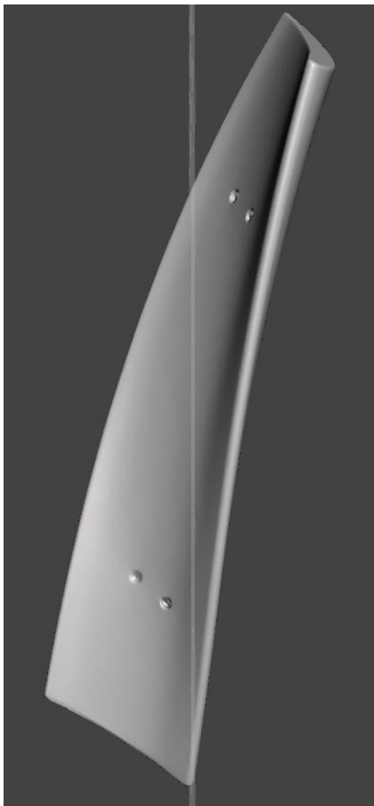
Figure 3-3: Scan of Darrieus blade
