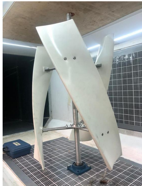
Figure 3-2: VAWT with Darrieus component only considered for this project
