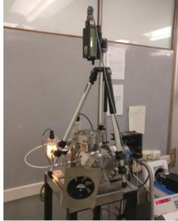
Figure 2.10: furnace for annealing in vacuum.
