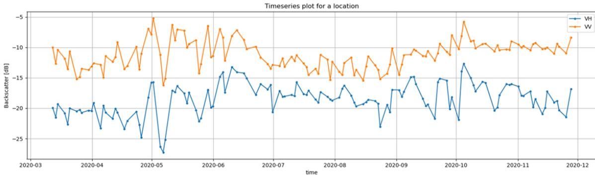
Figure 3.4:  $\sigma_{VH/VV}^0$  time series graph for a random rice pixel, before temporal-filtering and orbit-correction.
