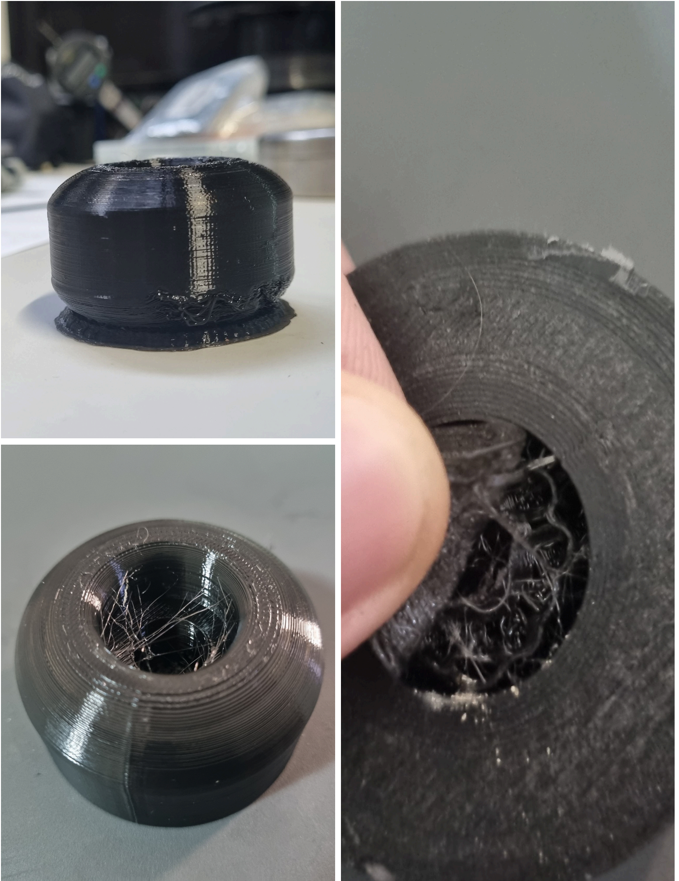
Img. 91 - Support flaw, retraction flaw and support removal, picture by the author.
