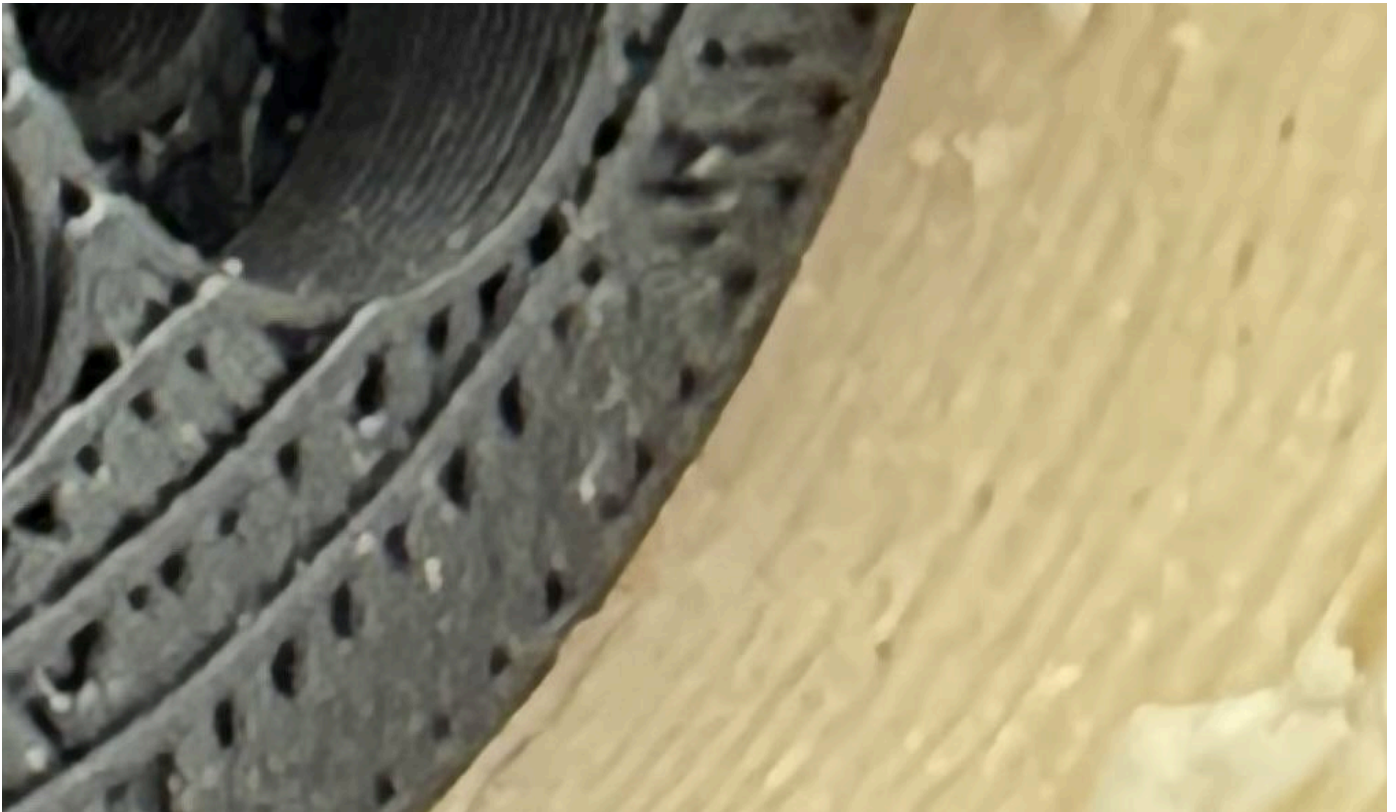
Img. 127 - Printing material detail (Nylon in black / biodegradable TPU in beige), picture by the author.
