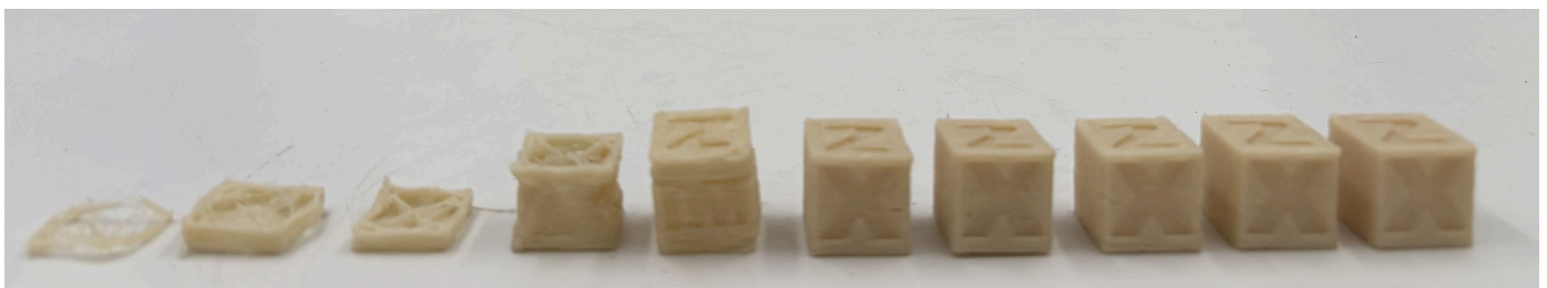
Img. 135 - Material (Ballena.filaflex) calibration, picture by the author.
