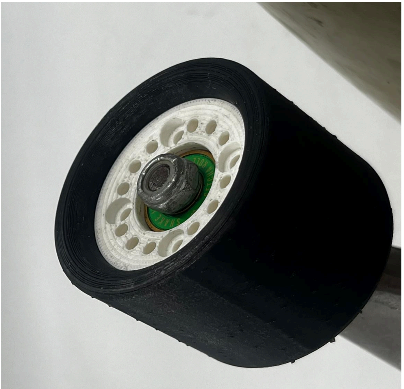
Img. 120 - Bearing insertion test + spin test documentation, picture by the author.
