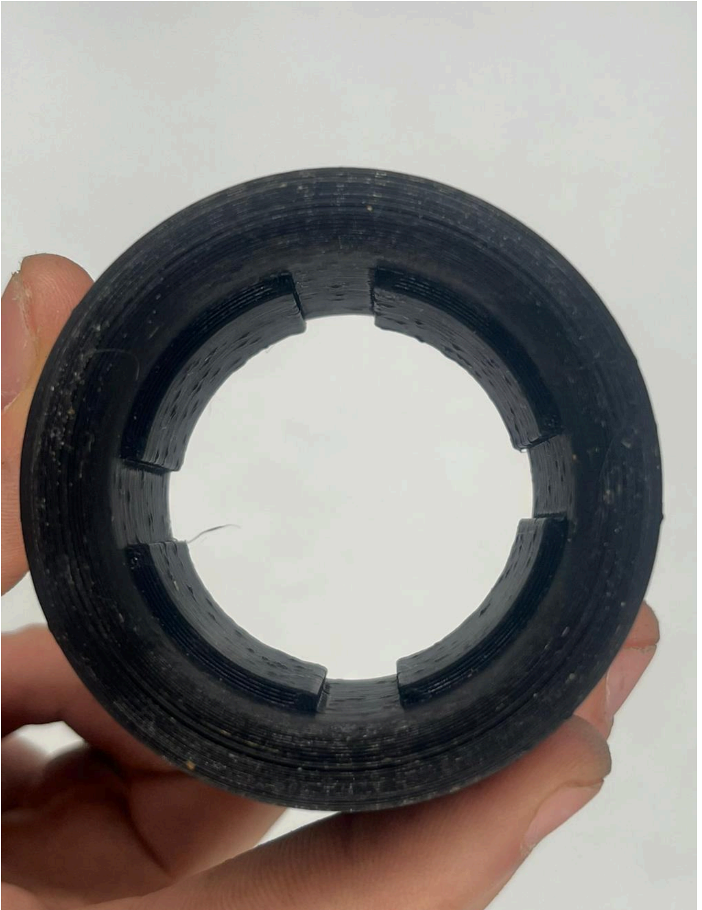
Img. 116 - Prototype of V2 (TPU tire), picture by the author.
