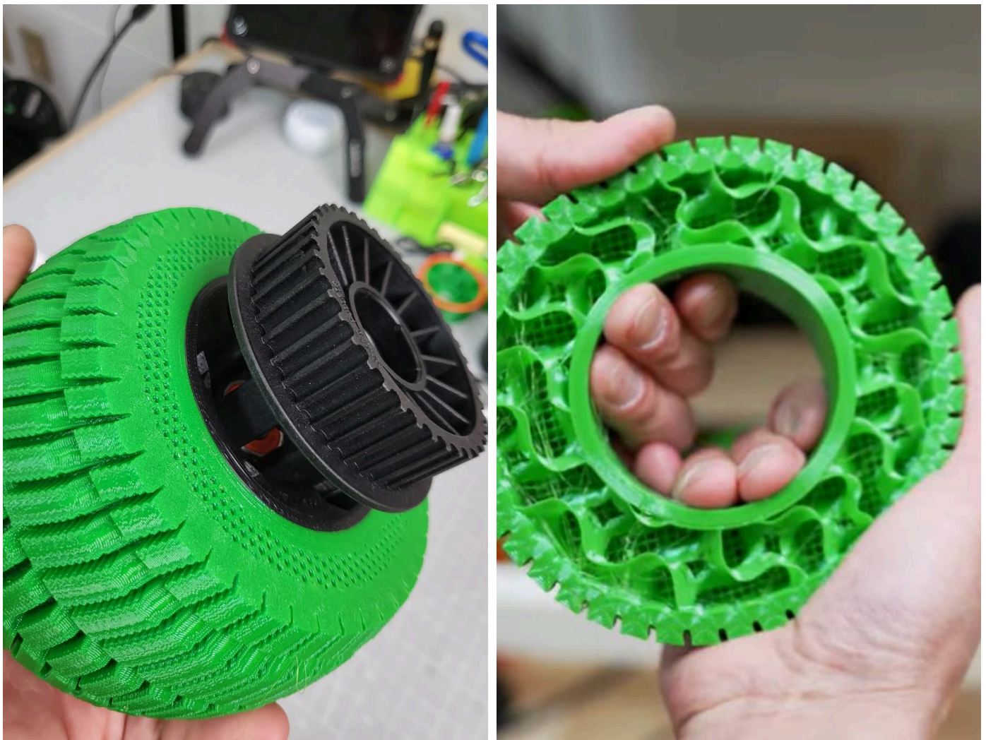
Img. 63 - 3D printed TPU wheels assemblage and section, by Dr. E.
