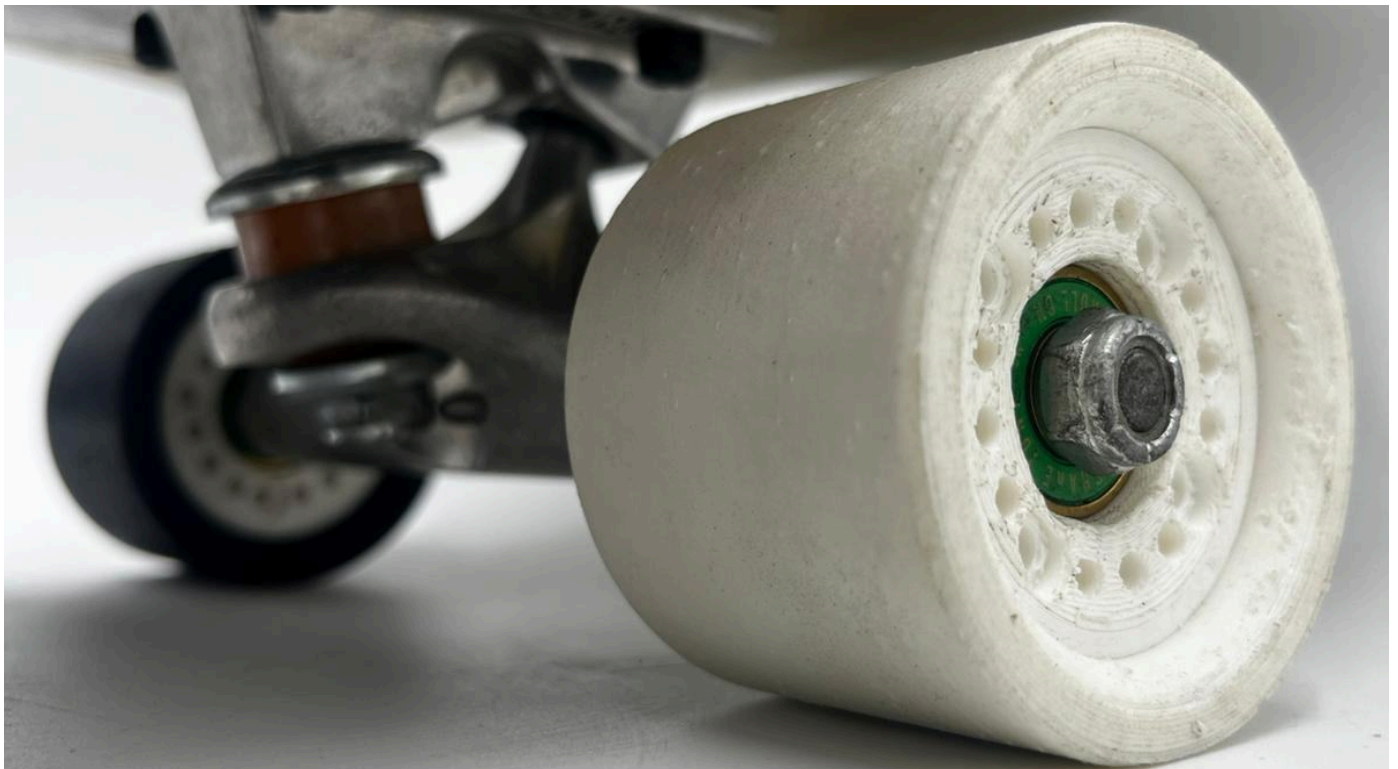
Img. 124 - Prototype tread using Filaflex Foamy, picture by the author.
