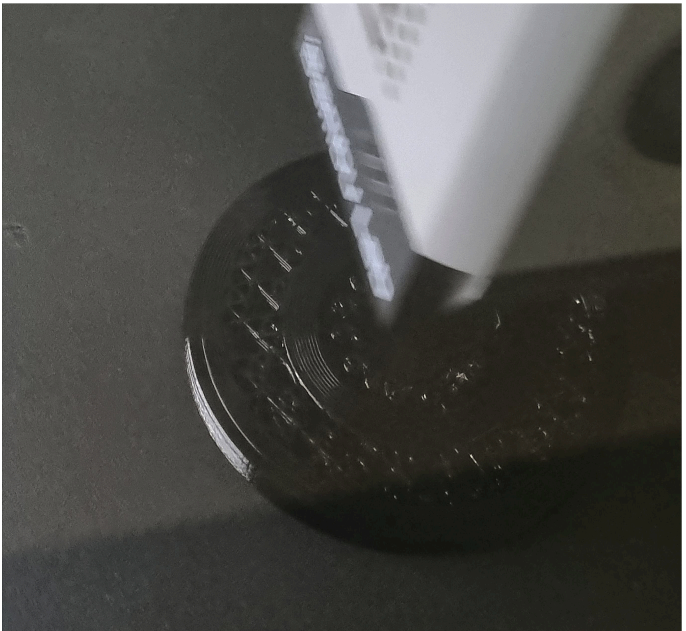
Img. 81 - Additive manufacturing of a wheel, picture by the author.
