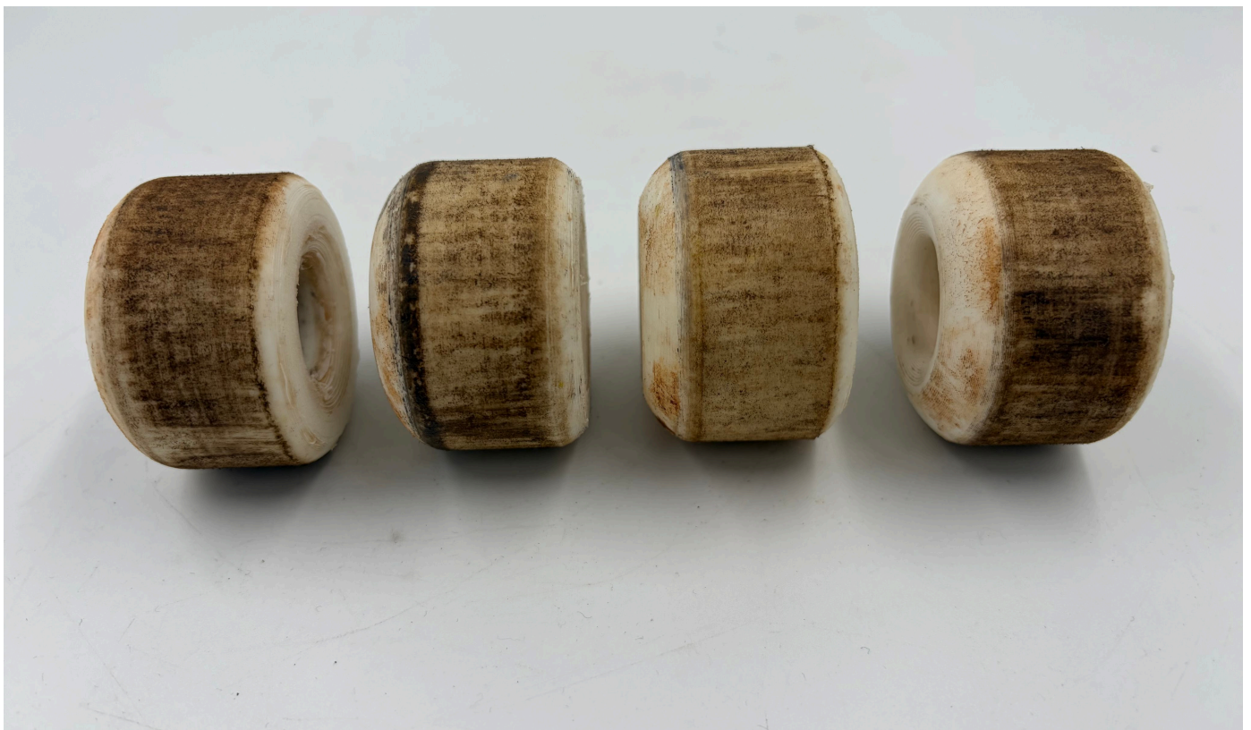
Img. 99 - Off-set wheel set 3d printed after use, picture by the author.
