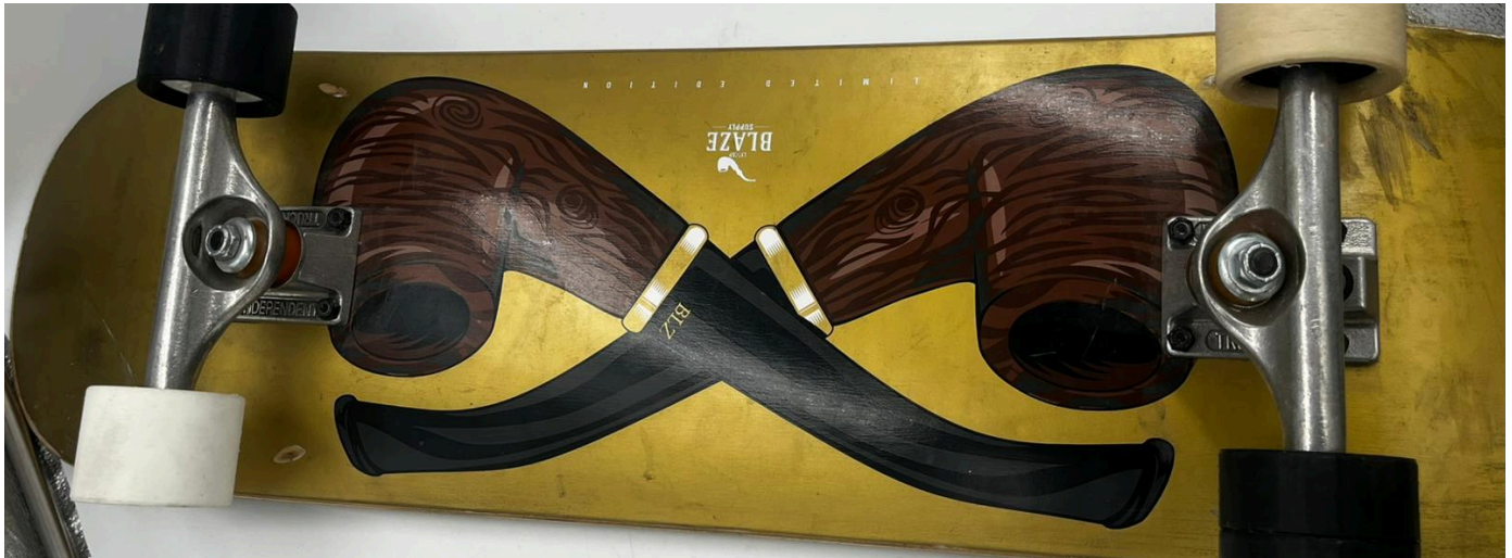
Img. 144 - Assembled 3D printed wheels on skate, picture by the author.
