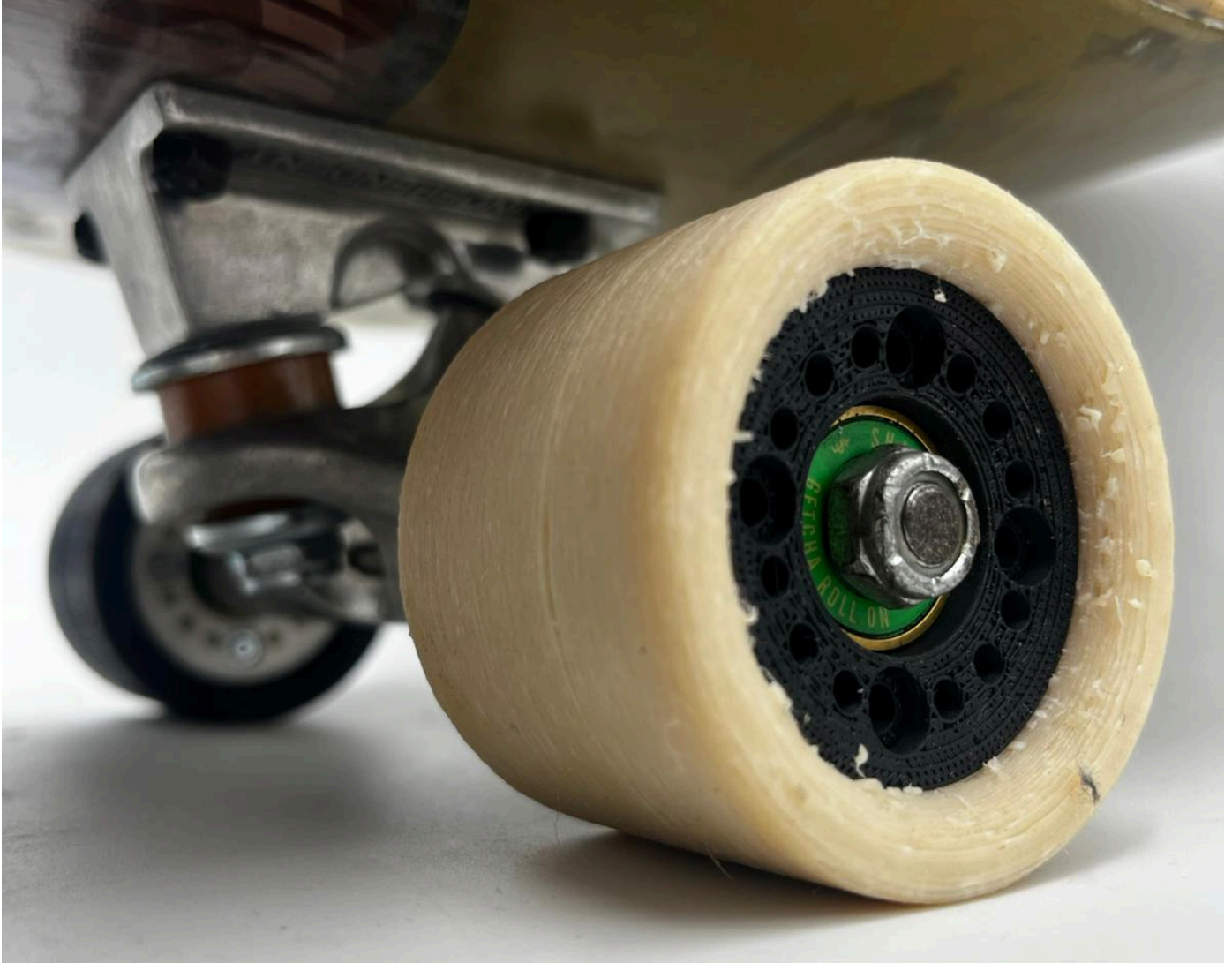
Img. 141 - Samsara Wheel assembled on skate, picture by the author.
