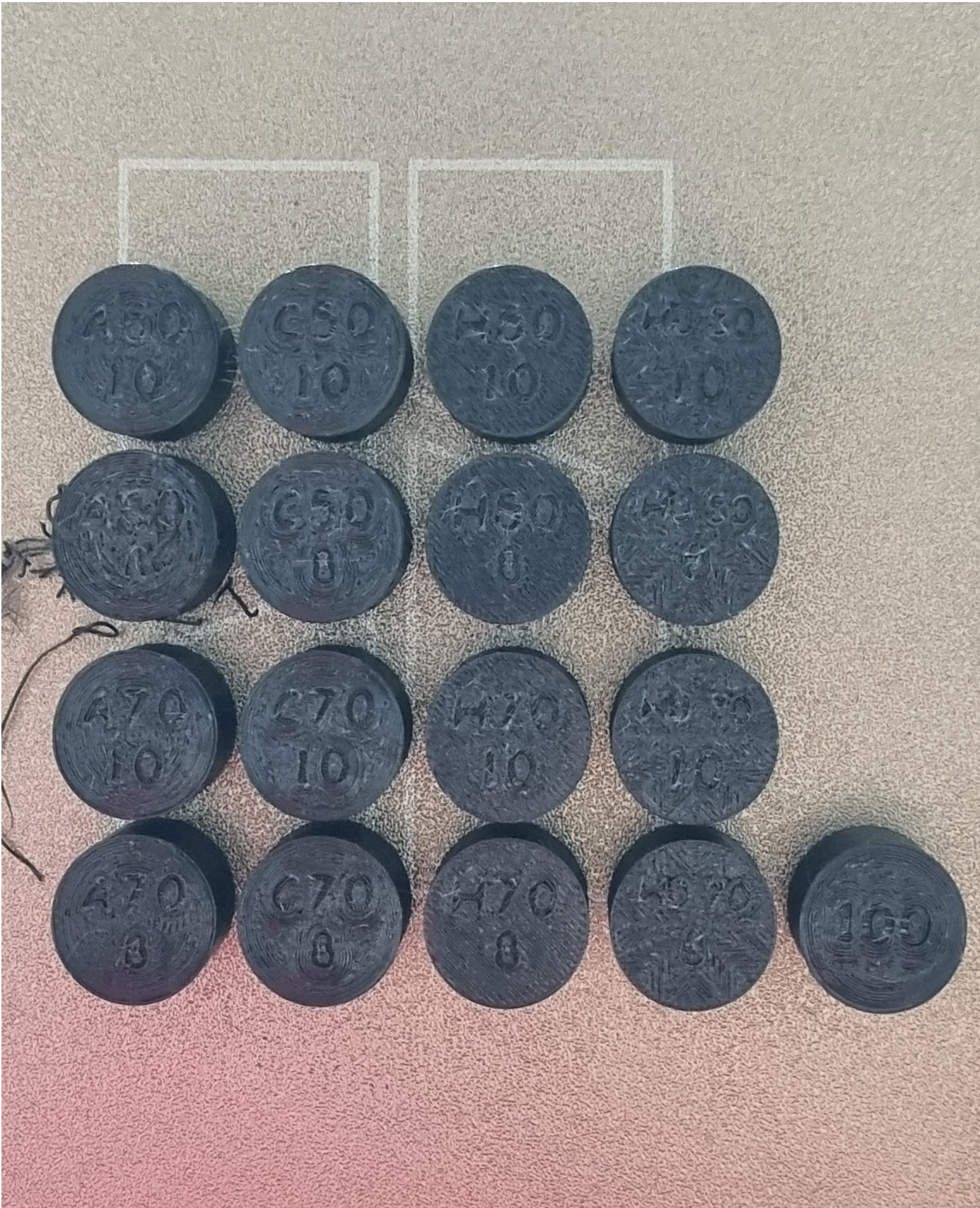
Img. 88 - 3d printed samples with different infill and wall thickness, picture by the author.
