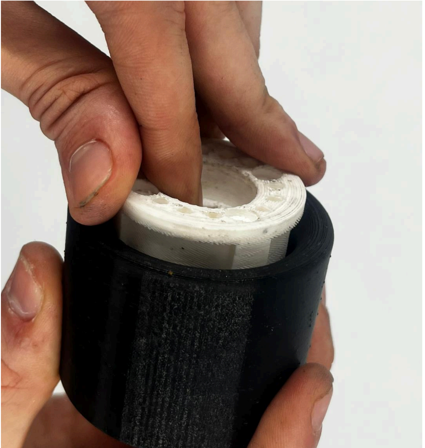
Img. 113 - Prototype of V2 (assembly by press-fit), picture by the author.
