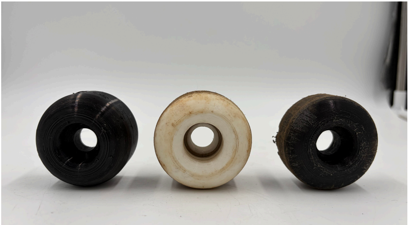
Img. 95 - Side-set, off-set and centered wheels 3d printed, picture by the author.
