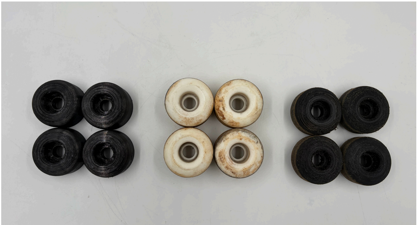
Img. 100 - Three sets of wheels 3d printed, picture by the author.
