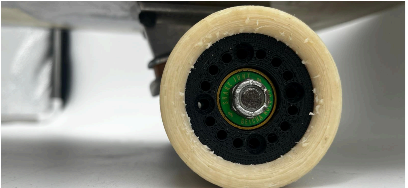
Img. 133 - Samsara Wheel assembled on skate, picture by the author.
