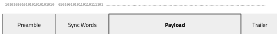
Figure 1.2.. General structure of a radio packet
