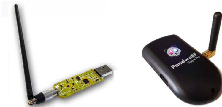
Figure 1.8.. A Yard Stick One [11] and a PandwaRF dongle [5]
