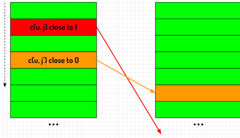
Figure 2.2.2: The two stacks represent the items sorted in descending order by the current model score, before (left) and after (right) the updates.
