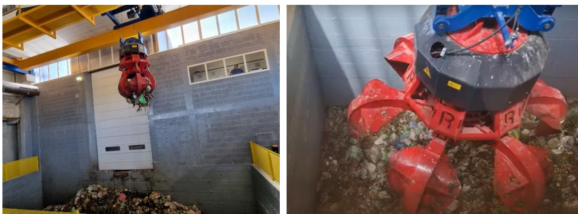
Figure 11: Polyp bucket crane.
