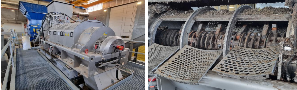
Figure 13: hammermill unit (left) with internal view of hammers and metallic screen (right).
