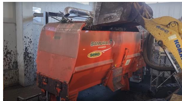
Figure 18: blender external view (left) with manual loading operations (right).
