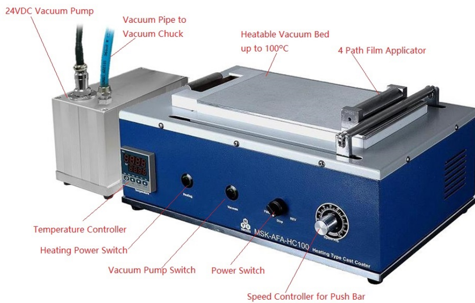
Figure 2.2: Tape caster with heatable vacuum bed and adjustable casting speed, picture from the supplier company MTI
