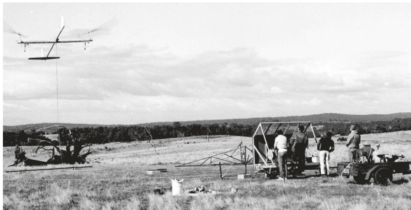
Figure 1.5: Test of the prototype created by the collaboration between Sky WindPower and Roberts. Photo taken in May 1986 [24].
