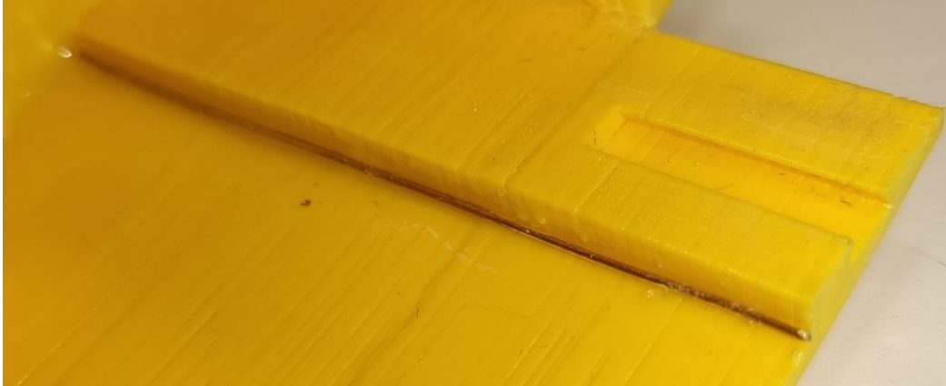
Figure 5.3: Brass wire reinforce, detail
