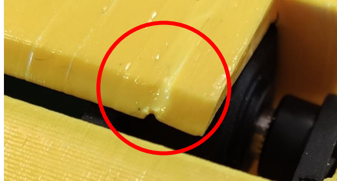
Figure 5.1: Filled crack in the shell
