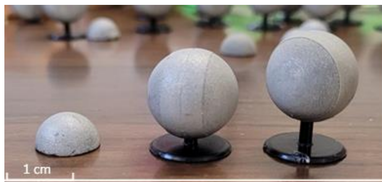
Figure 9: The three types of markers employed in the protocol.
