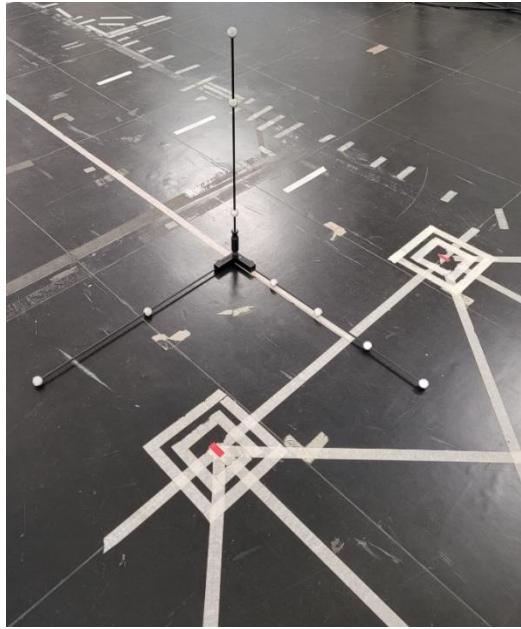
Figure 8: Cartesian triad used in the static phase of the calibration process.
