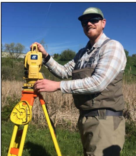
Figure 11: Total station with operator (48).
