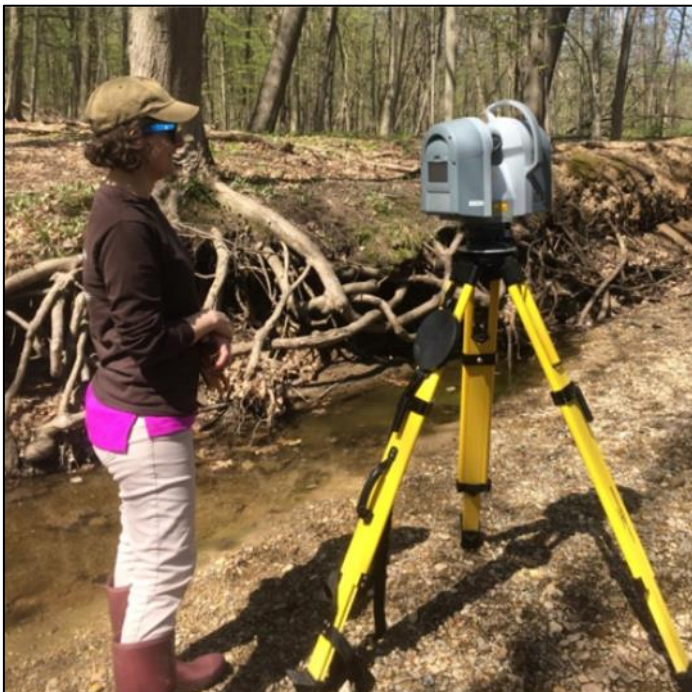
Figure 12: Laser scanner with operator (48).
