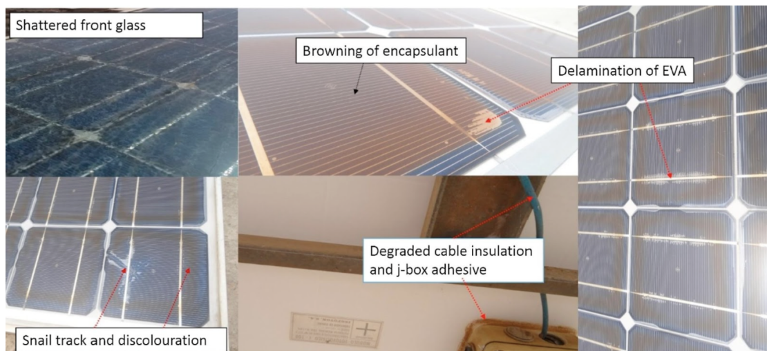
Figure 4.35: Ageing of PV modules
