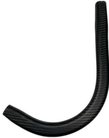
Figure 5.1: Preliminary prototype of the stick, without the optical fiber sensor
