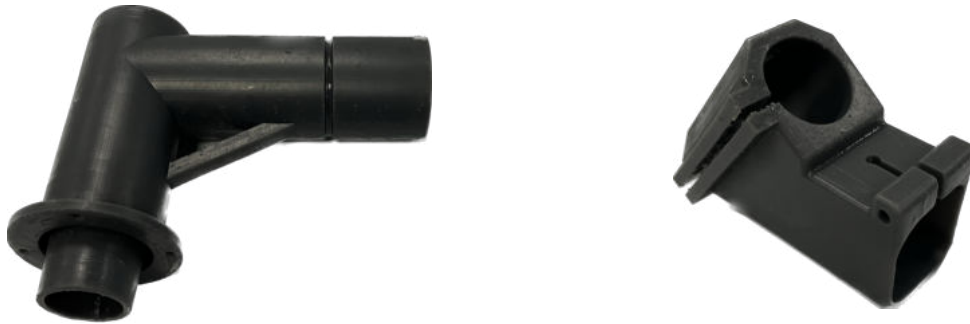
Figure 6.3: 3D printed grip for the load application (left) and stick-wall connection element (right)
