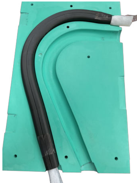
Figure 5.33: Mandrel closed with some tape
