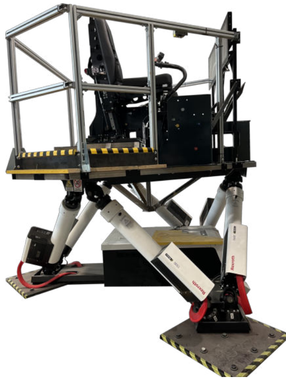
Figure 4.2: Motion Platform System (MPS) used as test-bed
