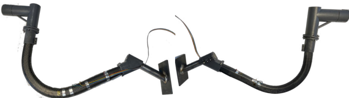
Figure 6.14: Strain gauges final setup
