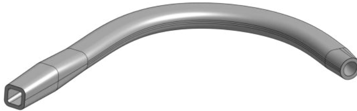
Figure 5.13: CAD of the hollow version of the mandrel
