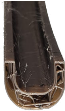
Figure 5.43: 3D printer pattern on the mandrel internal
