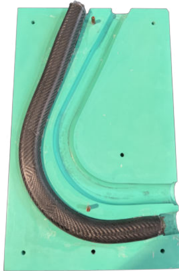
Figure 5.41: Stick after the autoclave cycle
