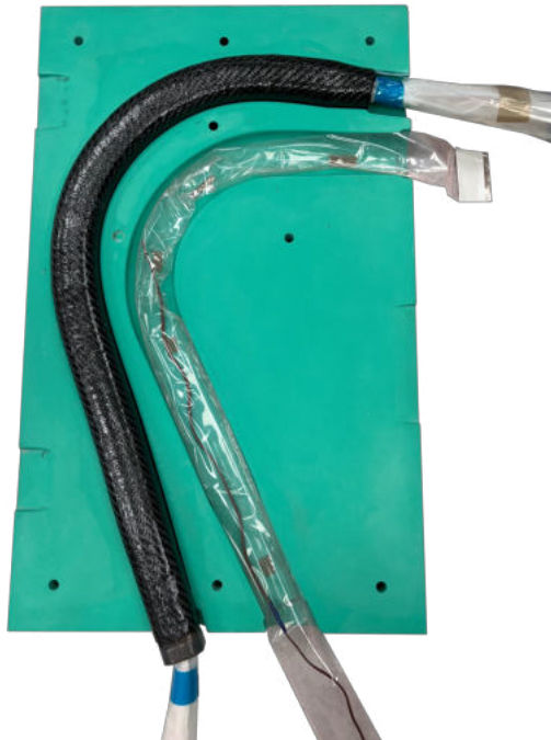
Figure 5.44: Tubular bag inside the mould empty cavity to solve the problem encountered during the autoclave cycle of the first stick prototype
