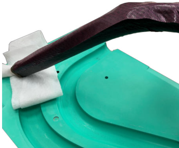
Figure 5.37: Particular of the wrapping procedure on the curved part of the mandrel
