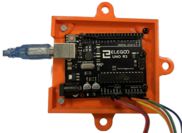
Figure 4.1: Arduino UNO microcontroller used for the OPT-IN sensors data acquisition
