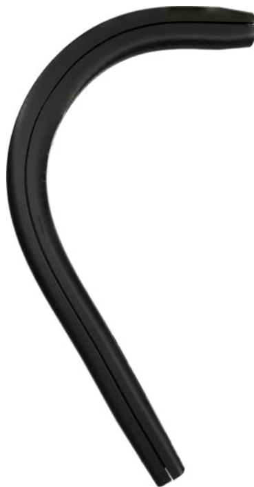
Figure 5.21: Matching of the two mandrel halves
