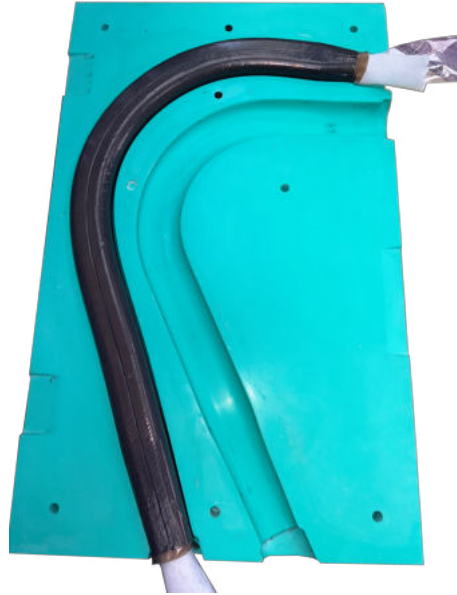
Figure 5.34: Mandrel with the teflon layer
