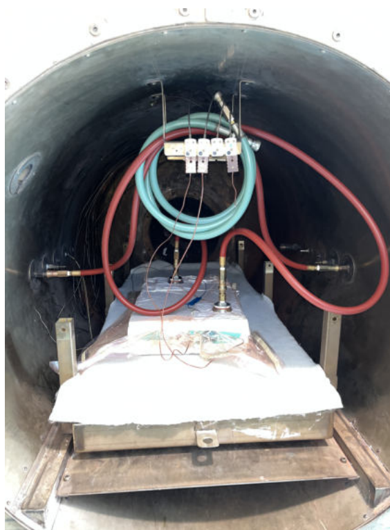
Figure 5.40: Vacuum bag inside the autoclave room
