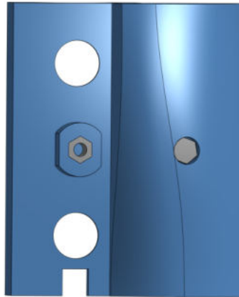
Figure 3.7: Connection of the inner and outer parts of the sliding portions of the grip
