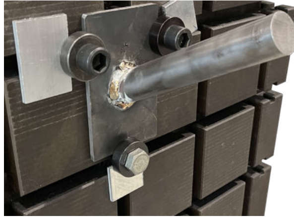
Figure 6.5: Test setup for the stick sensor calibration for the lateral force
