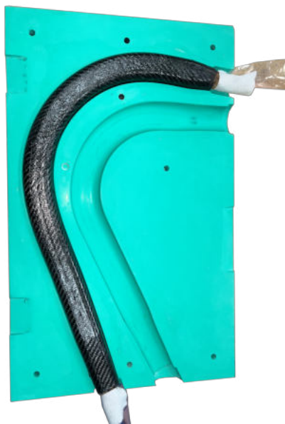
Figure 5.35: First pre-preg ply wrapped around the mandrel
