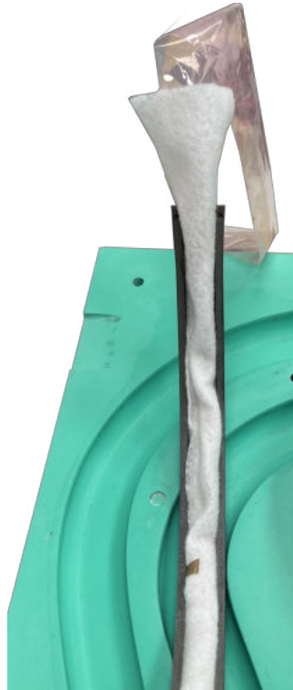
Figure 5.32: Tubular bag and breather layer inside the mandrel cavity
