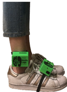
Figure 5.2: Two electronic boards placed over the foot of a diabetic subject to measure the exerted forces and the ankle joint angle.
