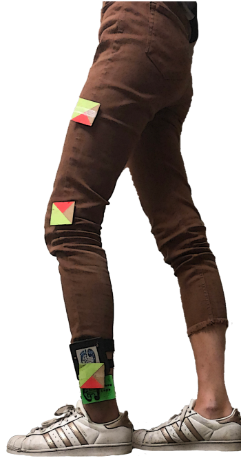
Figure 4.8: Comparison of the new MYLEG system and the original board in estimating the shank angle: experimental setup
