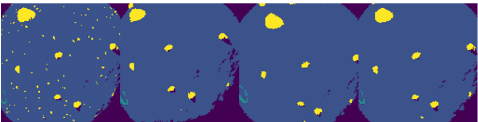
Figure 5.16: Comparison between the real segmented maps (Left) and the template ones with maximum correlations at the first three iterations. The correlation coefficient varies from left to right from 0.58, 0.69, and 0.75, while the error from 281, 111, and 21 m, respectively.
