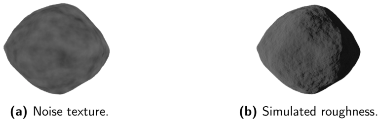
Figure 3.7: Surface roughness visualized on a model. Noise texture applied on the model (a). Displacement and bump on the model given by such texture (b).
