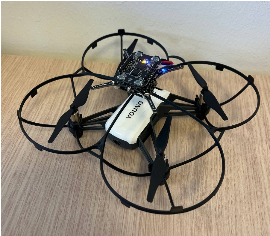
Figure 6.1: Hardware platform of DACS. The DJI Tello quadrotor provides actuation and visual sensing, while a Bitcraze Crazyflie 2.1 equipped with a Lighthouse positioning deck is rigidly mounted on top of the drone and supplies accurate indoor localization.
