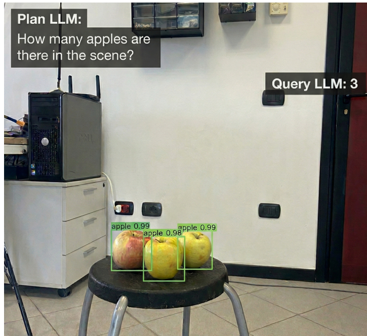
Figure 5.3: Example input output interaction of the Query LLM instance in DACS. The input includes the current camera image, the list of objects detected by the YOLO based Vision Encoder with their bounding boxes, and a natural language query such as “ How many apples are there in the scene ”. By jointly reasoning over the symbolic detections and the visual content of the image, the Query LLM instance produces a concise answer, in this case an integer count of the apples visible in the scene.
