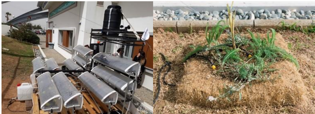
Figure 8-18: (left) Mangrove Still (MS) system in Akrotiri; (right) LifePatch with plants irrigated by water produced by MS system.
