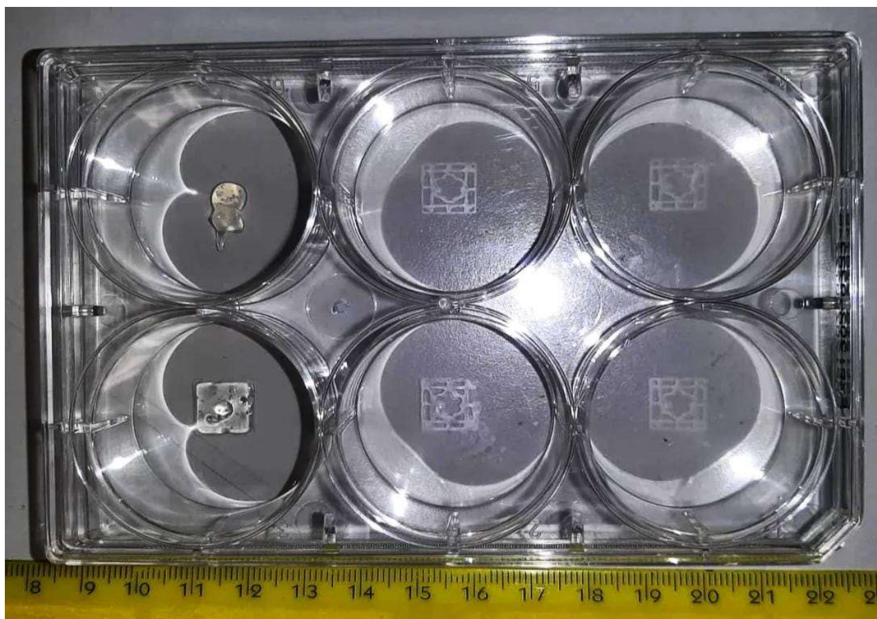
Figure 3.21 Grids printed using GelMA C bioink mixed with H5V GFP cells
