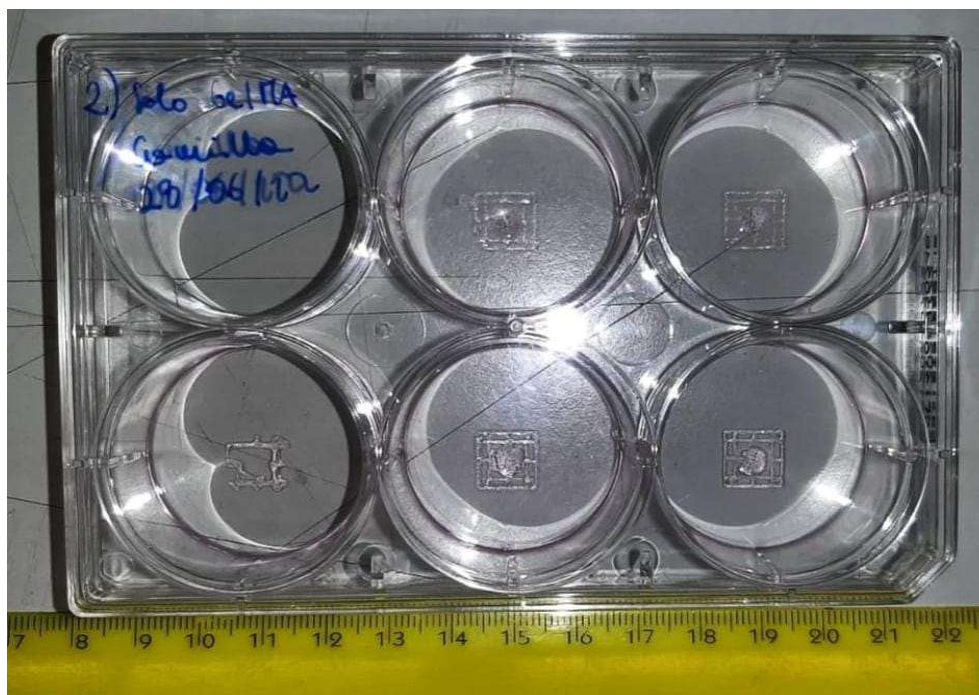
Figure 3.23 Caco2 cells-laden Matrigel droplets dispensed inside the grid holes
