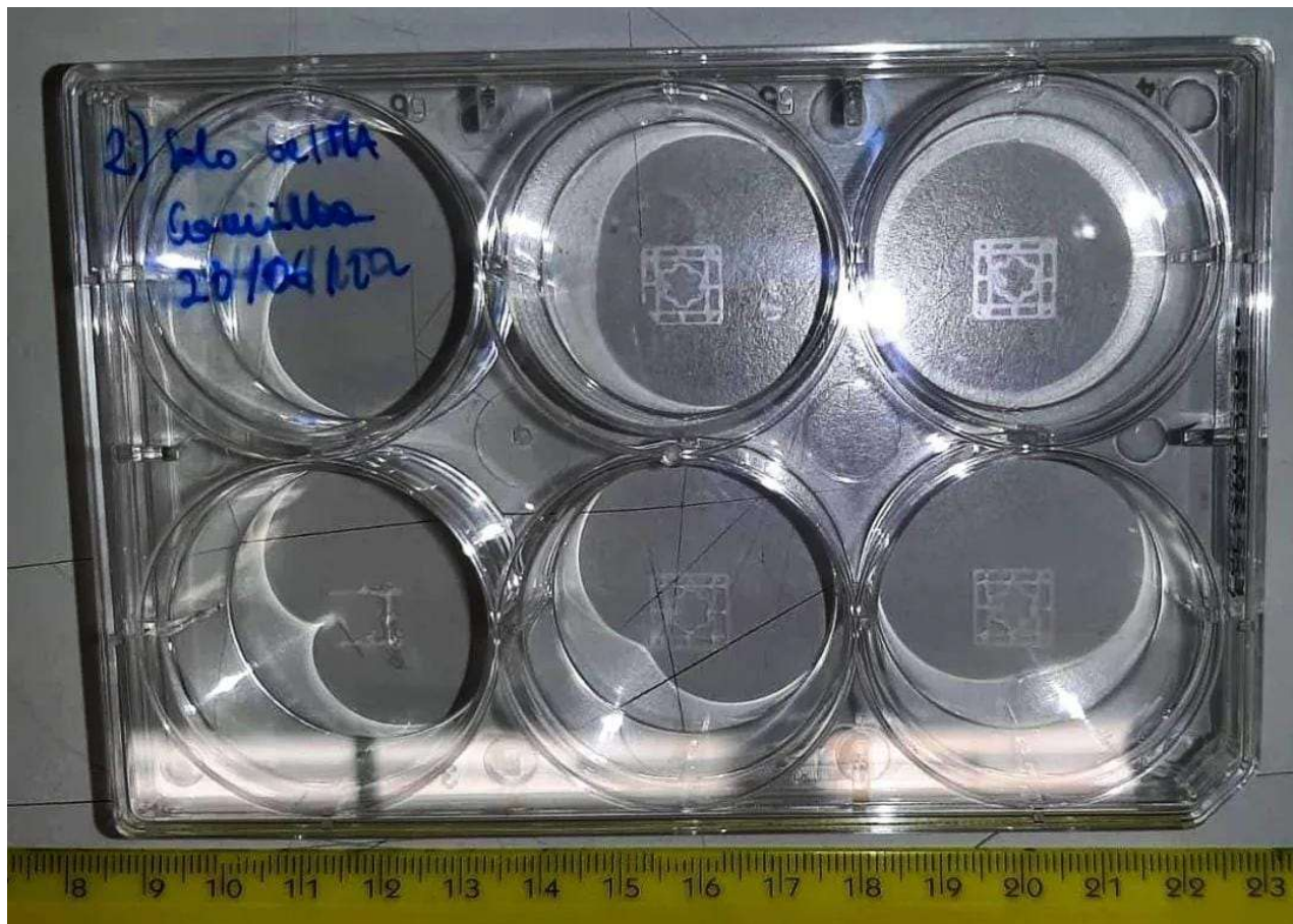
Figure 3.22 Grids printed using GelMA C bioink alone
