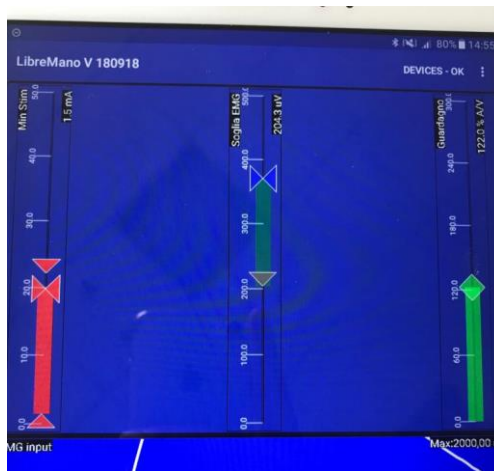
Figure 2.5 Application interface. the slider on the right modulates Gain, the one in the center the amplitude of the stimulation and the one on the left limits the maximum stimulation. the EMG of the recorded signal is shown below
