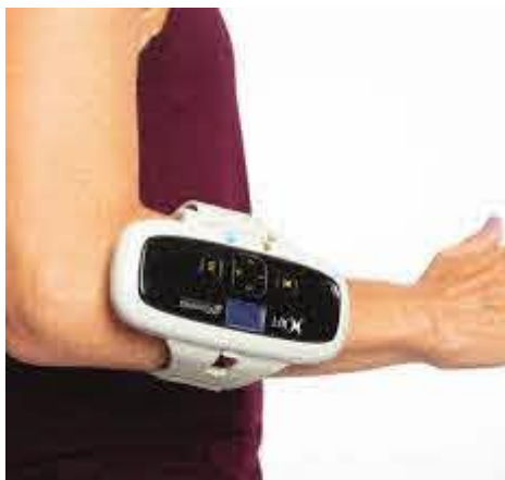
Figure 2.2 The OmniHi5™ Advanced FES Upper Extremity Treatment System [23] is a wearable functional electrical stimulation (FES) system for the upper limb which, thanks to an integrated electromyographic sensor, is activated by the intended movement of the user.
