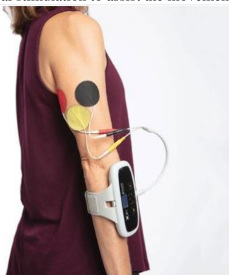
Figure 2.3 OmniHi5™ placement of hydrogel electrodes to use EMG control of FES.
