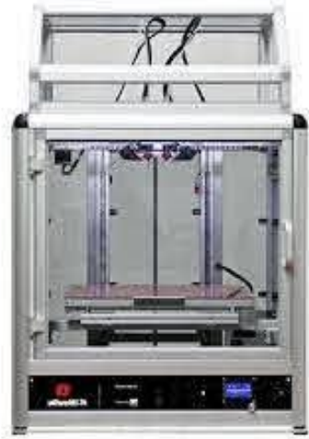
Figure 2.8 Olivetti s2 printer [36]. Above the printer are visible the extruders inside which the filament will be inserted. the print bed is in the rest position and will move closer to the extruders during printing
