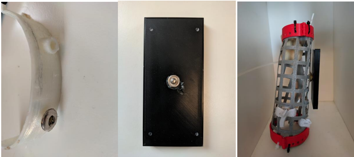
Figure 3.25 Assembly the electronic box with the TPU cage. From the left image there is the placement of the female part of the button in its seat (of a TPU printing test), the male part of the button placed in the center of the electronics box, the box assembled on the TPU part of the old prototype.
