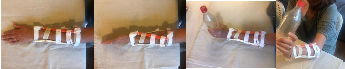
Figure 3.9 First prototype worn, it's shown the range of motion allowed by the prototype. A collaborator was asked to wear the device, perform prono-supination, grasp a bottle and approach it to the mouth by flexing the elbow
