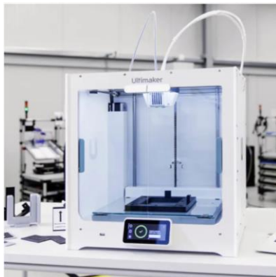
Figure 2.9 Ultimaker s5 [37]. Above the printer is visible the tube for the filament extrusion at the end of which there are the extruders. the print bed is in the rest position and will move closer to the extruders during printing
