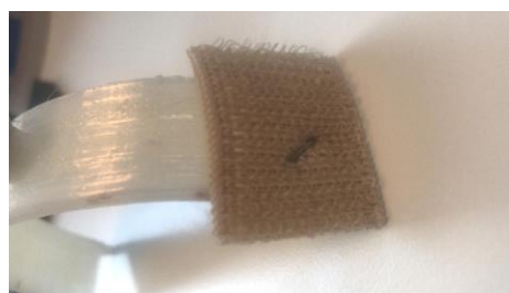
Figure 3.26 Test to evaluate the possibility to fix the Velcro band on the TPU part with the stapler.
