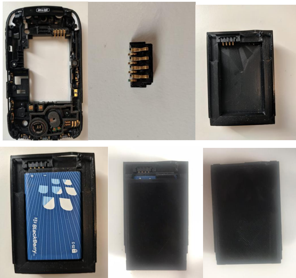
Figure 3.24 Battery box assembly process. From the first image on the top left there's the BlackBerry dismembered, the connector extracted, the connector placed on its seat in the battery box, the battery placed in its seat in the battery box, the lid in open configuration and the lid in closed configuration
