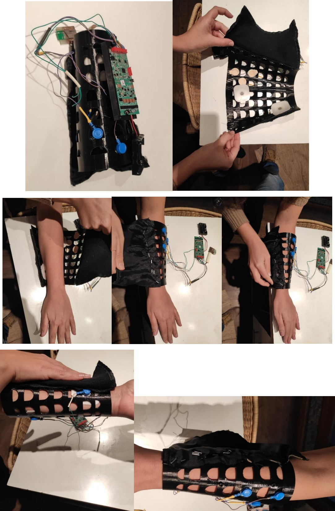
Figure 4.19 from the top left is show the assembly of the device with the MeCFES prototype, the open configuration with the placement of the electrodes subject specific, the wearing phases and the twisting of the forearm.
