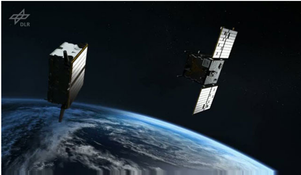
Figure 4.4: Image showing the two spacecrafts of the PRISMA mission: Tango (left) and Mango (right). Image from [44].
