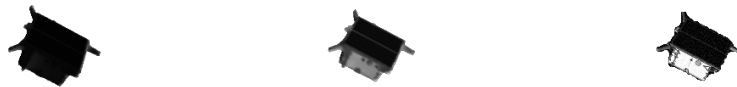
Figure 6.2: Rendering of the model before (left) and after (center) the pose adjustment step. The image on the right is the ground truth image. Result on the 6D vector representation. Starting IoU loss: 0.2453; final IoU loss: 0.0458; image name: img000014.jpg.
