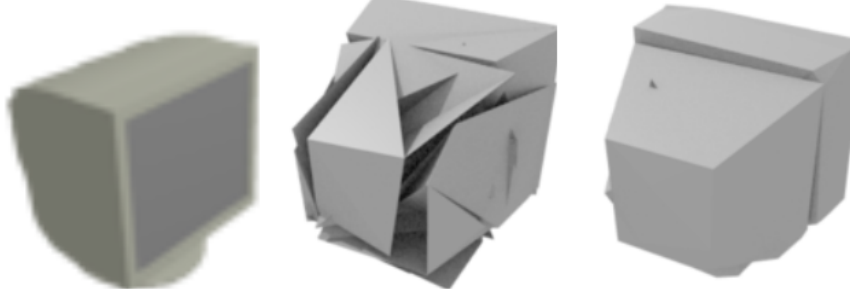
Figure 3.4: In this figure from the paper Kato, Ushiku, and Harada [18] is shown the effect of the smoothness loss on the reconstruction of a CTR monitor. Left: target image, middle: model predicted without smoothness loss, right: model predicted with smoothness loss
