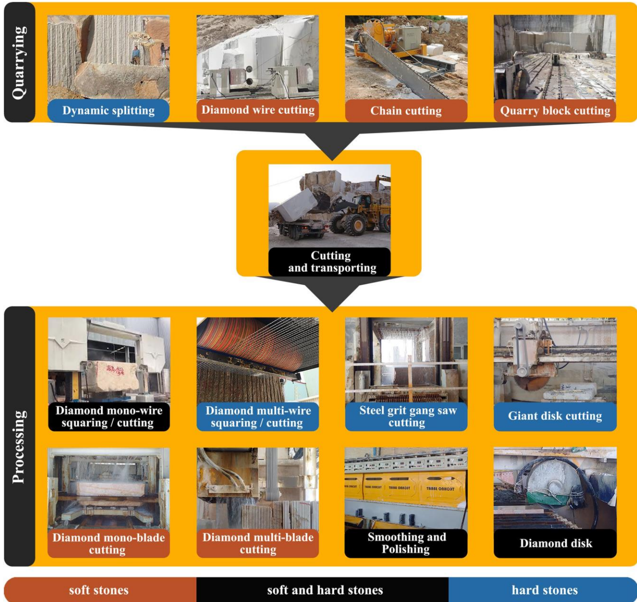
Fig 2.3-9: Quarrying and processing of dimension stones[52]
