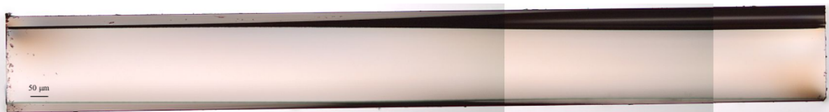
Figure 4.12. Cross sectional side view optical microscopy images of Y-splitters in OG diamond.
