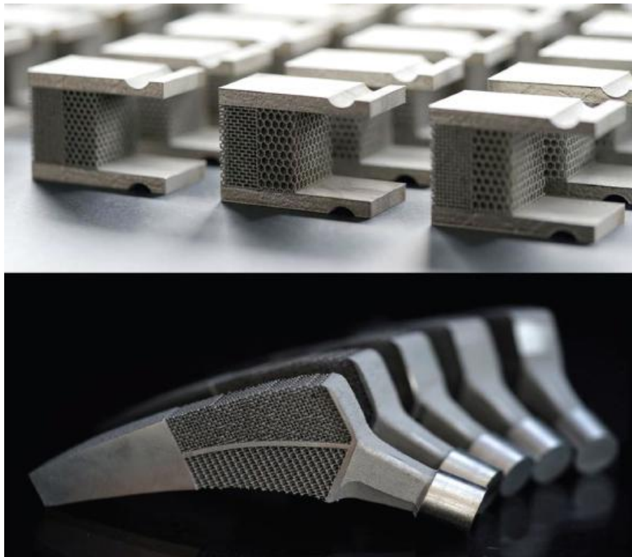
FIGURE 1.7.7 Combination of conventional and auxetic material (top) which leads to peripheral compression around hip stems (below) [53]
