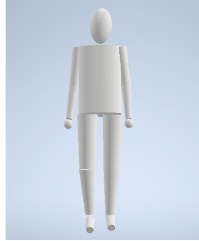
Figure 2: Reproduction of the 14-segmental geometrical model of the human body in CAD
