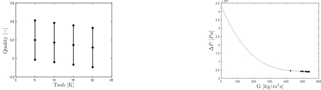
Figure 3: Error propagation of the vapor quality at the exit of the heater at P=7 kPa, and power=250 W
