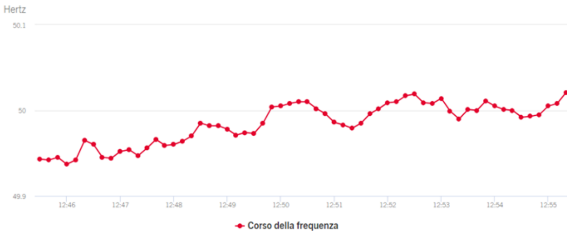
Figure 1.5: Snapshot of the frequency plot taken online in the moment in which this part was written.
