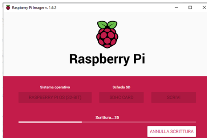
Figure 5.7: RPiImager: allows to write OSs on a SD card both suggested by the software or downloaded by internet.
