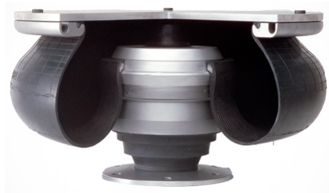
Figure 3.13: Air spring for the secondary suspension of railway vehicles
