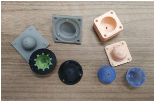
FDM printed moulds and molded parts [u]
