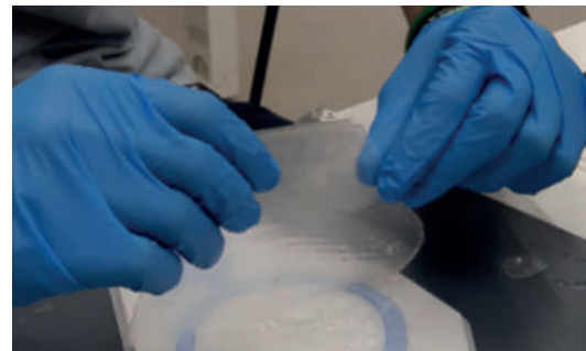
[Z] silicone casted layers and sandwich bonding
