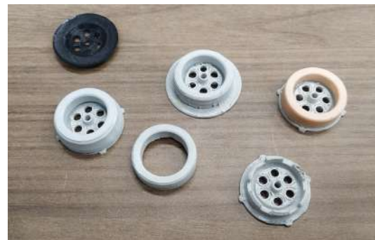
[S] FDM functional printed parts
