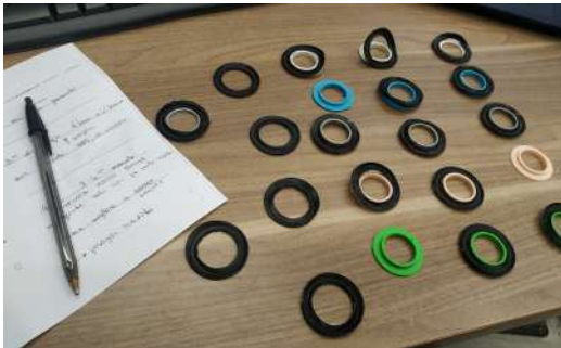
results of material welding tests
