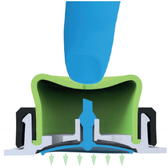
opened valve - low cracking pressure (inflation)
