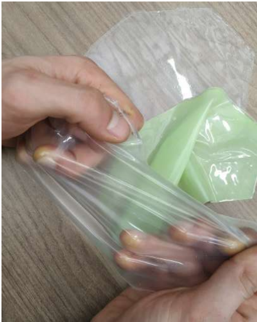
self-made silicone sheets (0,6-0,2 mm thick) [F]
