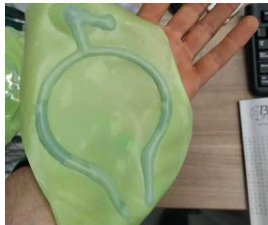
[H] picture showing silicone inflated circuit
