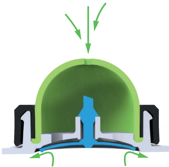
closed valve - high backward pressure (deflation)
