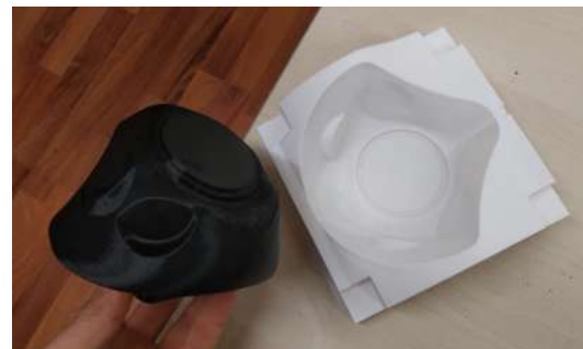
[Y] FDM functional printed parts
