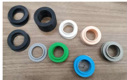
[T] different materials FDM printed samples
