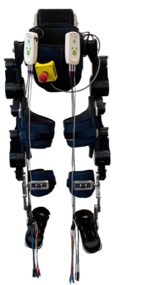
Figure 1: TwinFES prototype consisting of the Twin exoskeleton and two electrical stimulators
