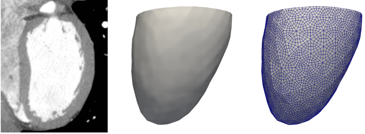
Figure 1.2: Example of computed tomography scan of a left ventricle (left), the Zygote Solid 3D model [Inc14] (center) and a corresponding mesh with 36704 elements (right). The CT scan has been taken from https://images.app.goo.gl/SGUuFVAQ8RxyDbsw7 .
