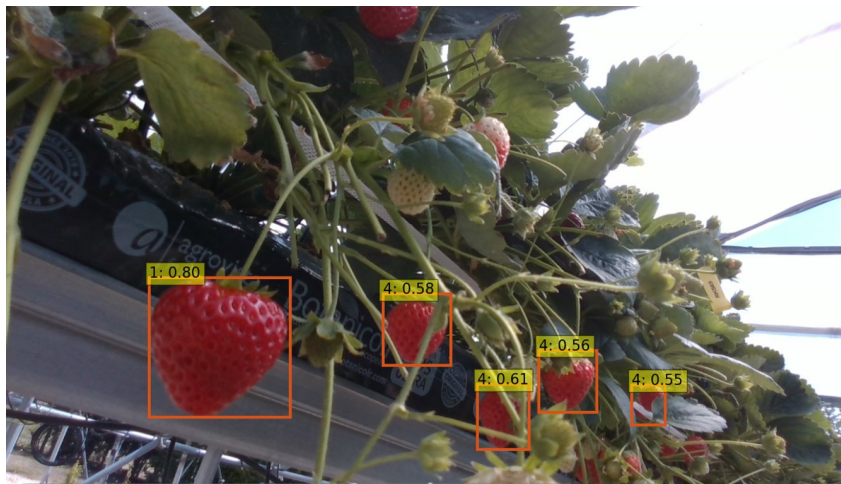
Figure 4.3: Fine-tuned DETR output: strawberries identification and scheduling identification. The integer numbers represent the predicted order of picking, the other number is the probability of the prediction
