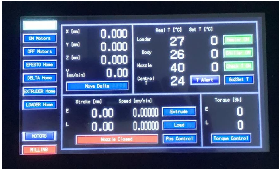
Figure 69: HMI temperature control
