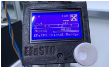
Figure 2: Display to control bed temperature and fan
