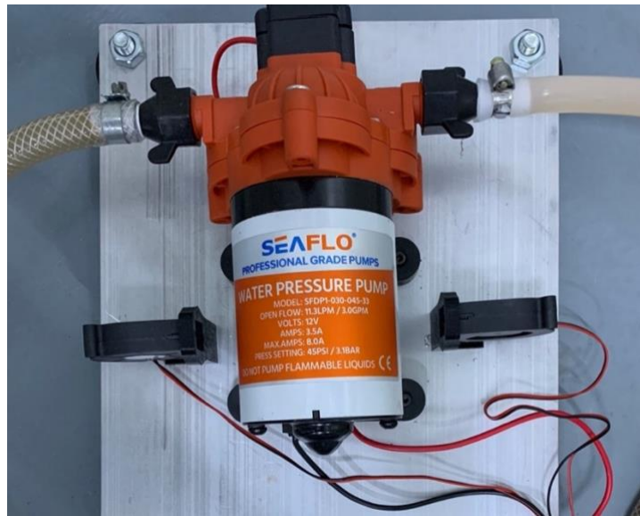
Figure 88: Pump structure with fans
