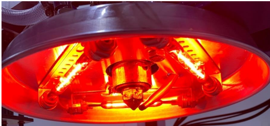
Figure 107: IR heater side view
