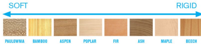
Figure 1.2: Wood used in the ski construction.
