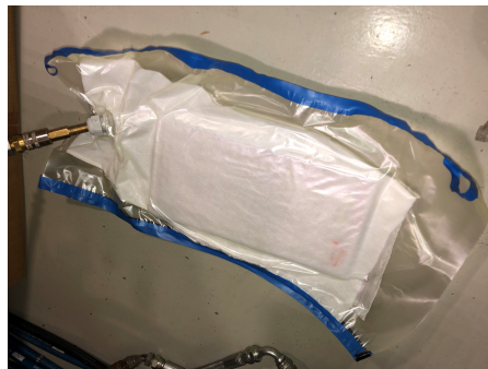
Figure 5.9: Vacuum bagging process.
