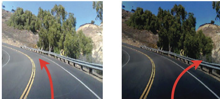
Figure 2.3: Left image is the original input image that correctly makes a decision result. The right image is the generated image which makes an error with respect to the expected result [45].
