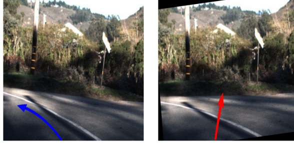
Figure 2.1: Blue arrow is the expected steering in original images and red arrow is the steering result with six-degree rotation [55].
